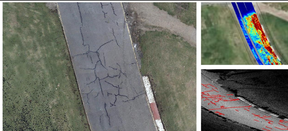
Figure 9: Example output from MLS and GPR for Pavement Analysis
