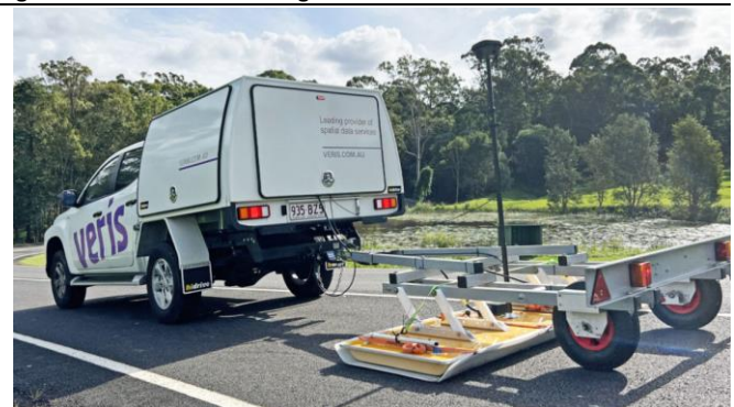
Figure 8: Ground Penetrating Radar Vehicle
